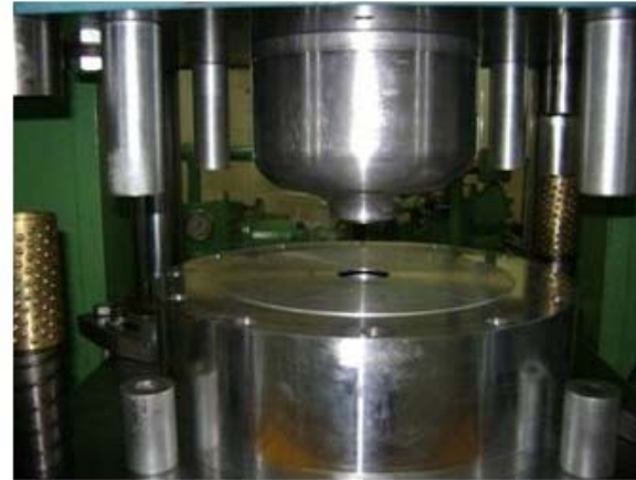
Blank Loading for Forming
