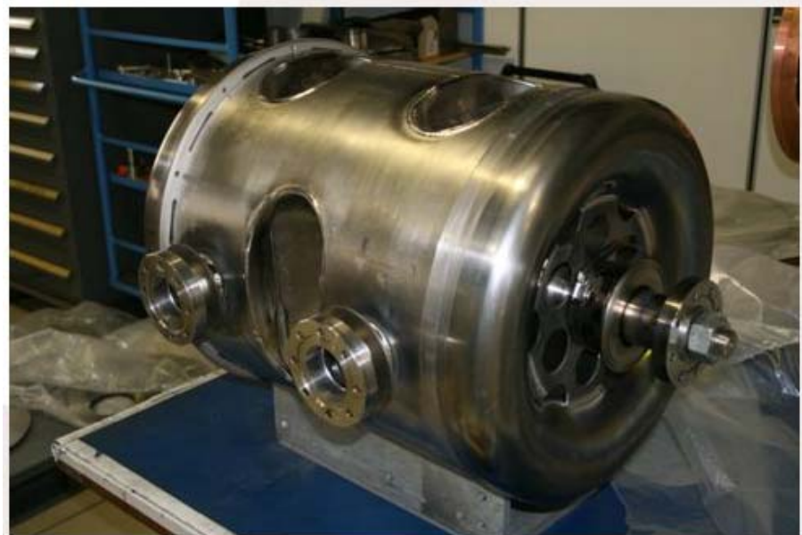
Typical spoke cavity
