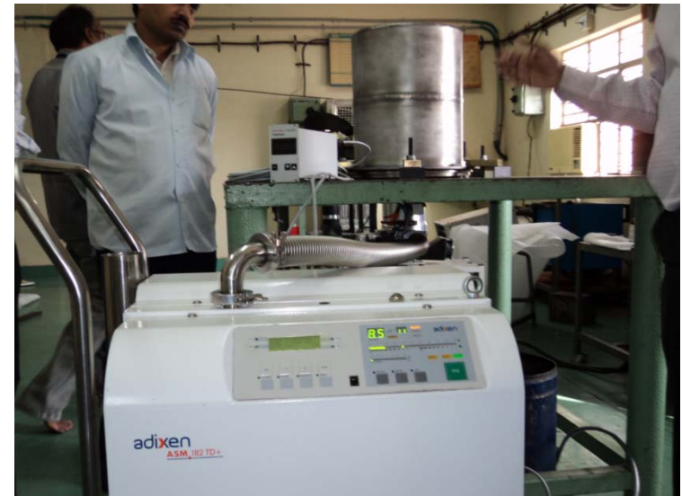
He vessel under He leak testing
