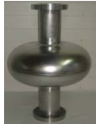
Laser welded single cell SCRF cavity Under inspection
