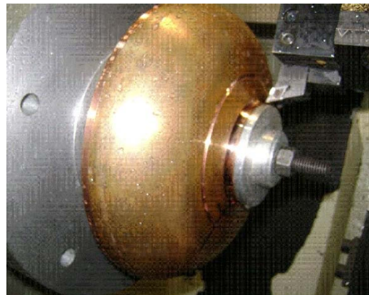
Machining of iris OD and shoulder
