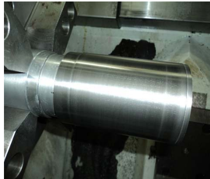
End pipe machining
