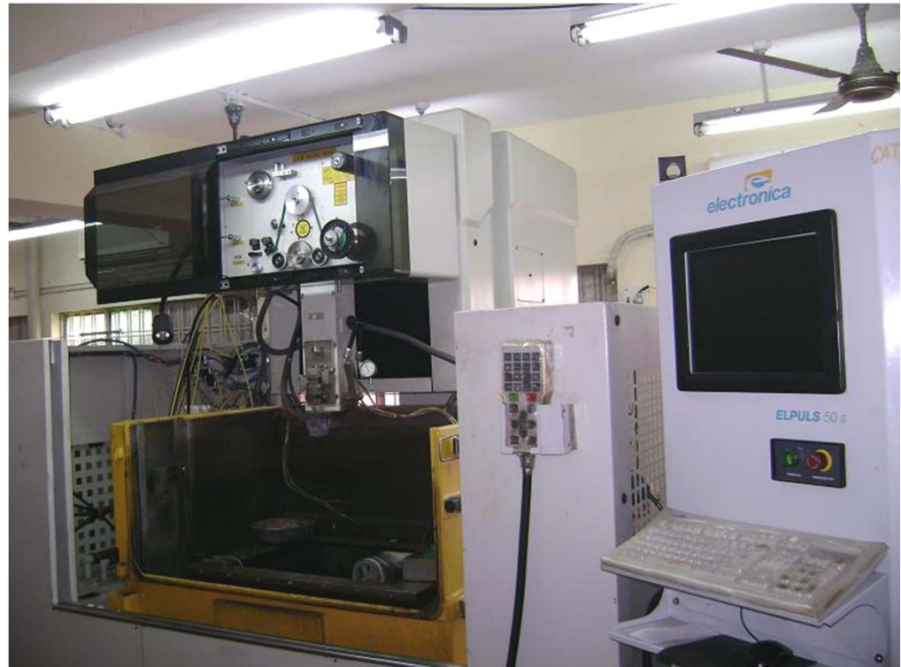
CNC EDM Submersed and Flush Type Wire Cut Machines X,Y & Z strokes-600, 400 & 400 mm Accuracies - \pm 10 \mu\text{m}
